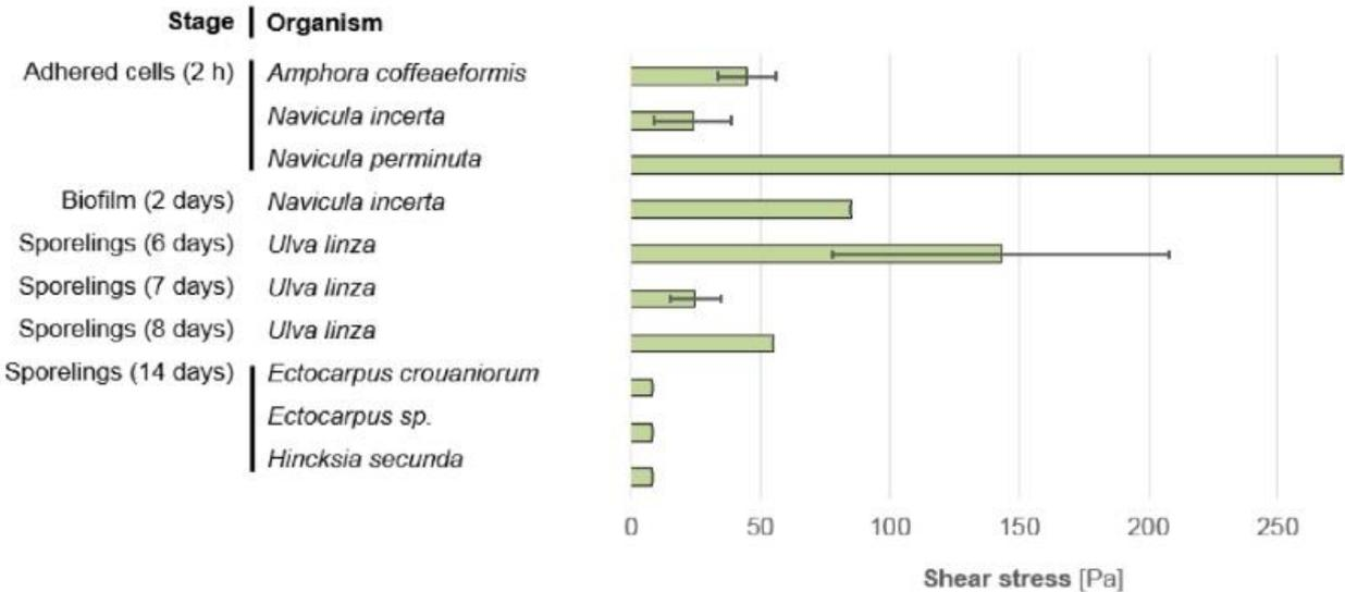
**Figure 1.** Forces needed for removal of microalgae and macroalgal sporelings from foul-release paint (based on literature values, graph from Oliveira and Granhag 2016).
