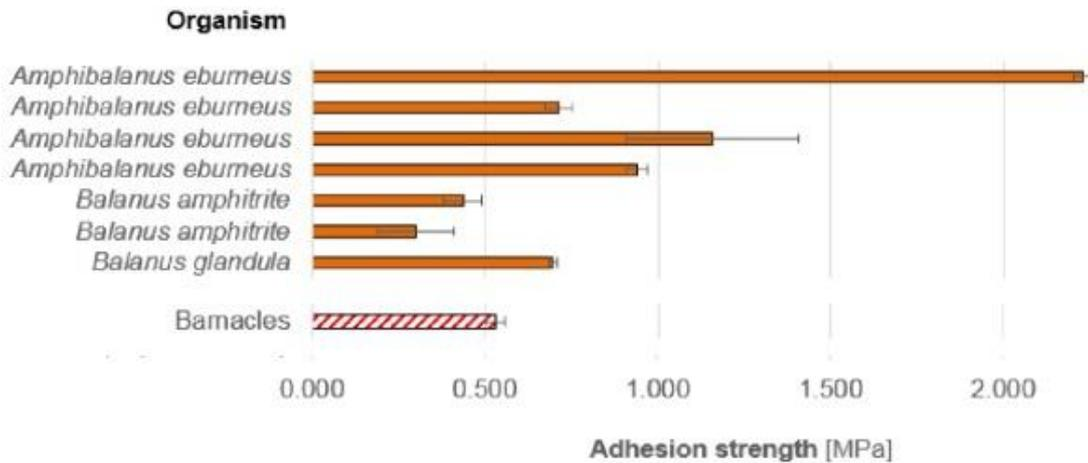
**Figure 2.** Forces needed for removal of different barnacles from hard paint (red) and self polishing coating (striped) (based on literature values, graph from Oliveira and Granhag 2016).
