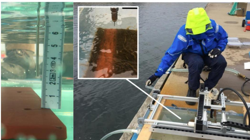
**Figure 4.** Waterjet device used in field experiment, waterjet nozzle (detailed figure to the left).
