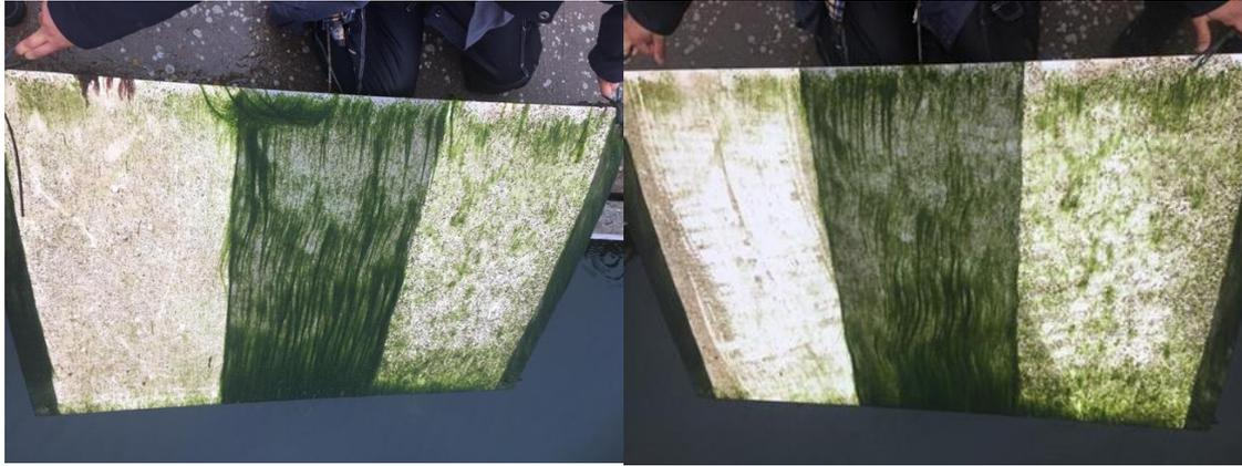
**Figure 7.** Field test panels deployed in Saltholmen marina July 2019, before and after cleaning, from left Ecopower Racing, Grey Primer (control) and Lefant T-coat.
