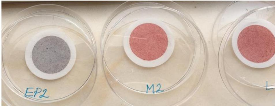
**Figure 6.** Paint particles from three leisure boat paints on filters.
