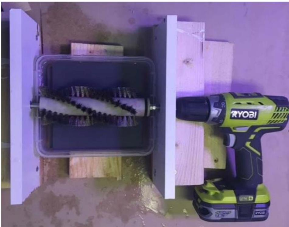
**Figure 5.** Setup for cleaning of in lab, with panels to be cleaned placed on bottom of container.
