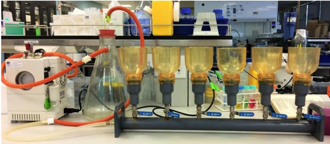
Figure 1: Six-way filtering system for lab-based filtering of water samples (photo: A. Zaiko).
