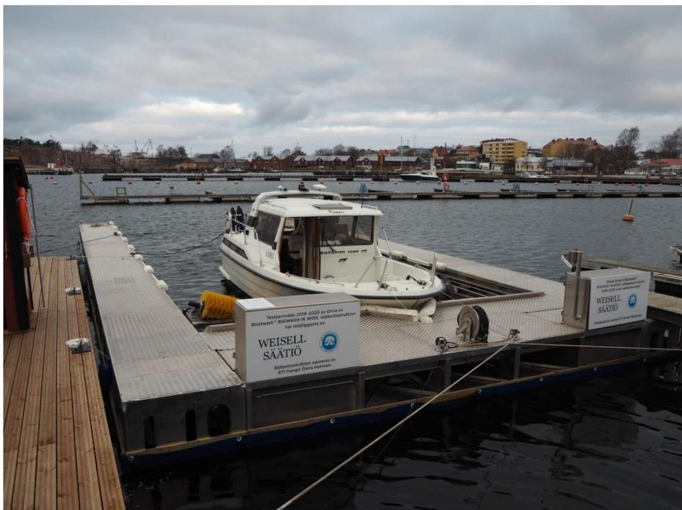
Figure 2. Drive-in boat wash for large recreational vessels such as sail boats. Photo: Keep the Archipelago Tidy
